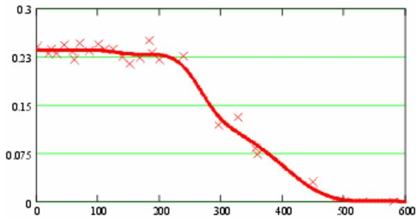
Figure 13:  $\delta_{\text{RGB}}$  as function of spatial frequency (LP/H) for the CFA-SLR. This loss of color at spatial frequencies above 300 LP/PH was typical of all digital cameras tested.
