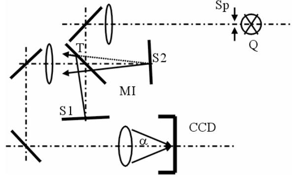
Figure 9 Diagram of the Michelson interferometer
