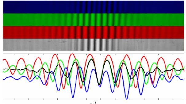
Figure 11: The interferograms for blue, green, and red channels as well as a combined luminance channel. The plot shows how the intensity curves differ.
