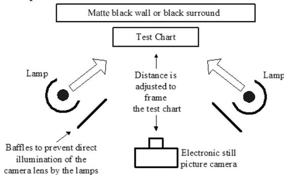
Figure 1: Setup for resolution target measurement as specified in ISO 12233.
