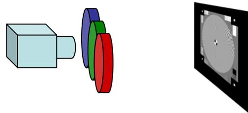
Figure 2: Blue, Green or Red filters are added between the camera lens and the resolution target to achieve color resolution measurements..
