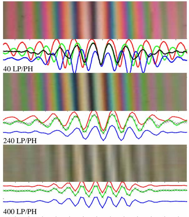
Figure 12: Images of white-light interferograms taken using a color filter array SLR digital camera. As the spatial frequency is increased, the color saturation decreases until all color information is lost. The colored curves that correspond to intensity in the RGB channels become the same.
