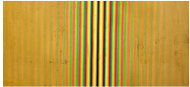
Figure 10: An example white-light interferogram from the Michelson interferometer. The fringe distance varies as a function of wavelength giving a color pattern useful for testing a camera's color resolution.
