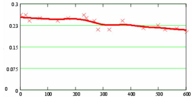
Figure 14:  $\delta_{\text{RGB}}$  as function of spatial frequency (LP/H) for the X3-SLR. The lack fall-off of color saturation with spatial frequency differs from other cameras tested.
